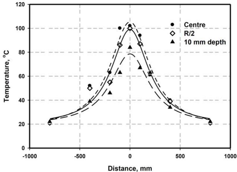
**Figure 3.** Temperature distribution along the log (diameter 128mm, moisture content 28%, oven dry density  $401\text{kg/m}^3$ ) after heating during 20 second in applicator (350A). MW power was supplied via 3 radiators each with 10kW of power, vector E orientation is parallel to the wood grain in all ports. 0 – plane of the radiator centre.
