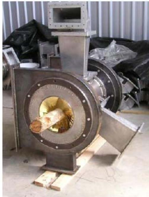
**Figure 2.** MW applicator (350A) for round timber with power supply to the applicator via three ports (radiators). (a) diagram, (b) MW applicator photo.
