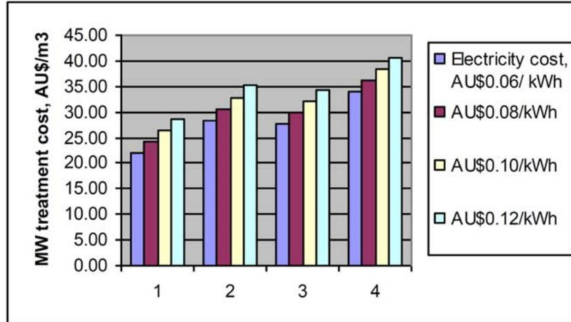
**Figure 5.** MW log processing costs depending on plant output and electricity costs (frequency 0.922GHz). (1) Automatic plant, three working shifts per day, output 24,000m<sup>3</sup>/year; (2) automatic plant, two working shifts per day, output 16,000m<sup>3</sup>/year; (3) one plant operator per shift, three working shifts per day, output 24,000m<sup>3</sup>/year; and (4) one plant operator per shift, two working shifts per day, output 16,000m<sup>3</sup>/year.
