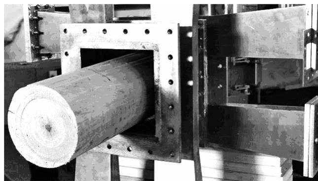
Figure 1.—Peeler core position on the PC-1 applicators.
