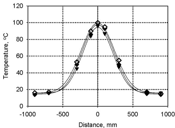
**Fig. 4** Temperature distribution along the sleeper (size  $130 \times 260 \text{ mm}^2$ , MC = 34%, oven dry density  $480 \text{ kg/m}^3$ ) after heating for 20 seconds in the MW applicator. MW power of 90 kW was supplied via 4 radiators (from top and bottom 25 kW each and 20 kW from every side, vector E orientation is perpendicular to the wood grain in all ports. 0—plane of the radiator centres)
