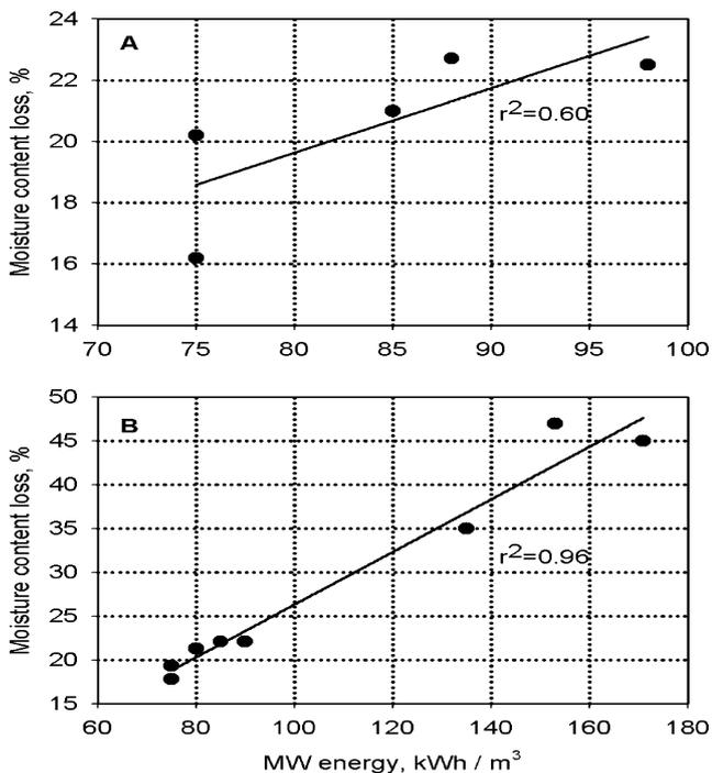
**Fig. 6** Sleeper moisture content losses depending on applied MW energy. (a) sleeper size  $130 \times 225 \text{ mm}^2$  and wood green density range  $570\text{--}730 \text{ kg/m}^3$ , (b) sleeper size  $130 \times 260 \text{ mm}^2$  and wood green density range  $650\text{--}690 \text{ kg/m}^3$
