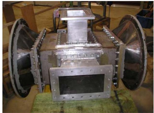
**Fig. 3** MW applicator for railway sleepers with power supply to the applicator via four ports (radiators). (a) Diagram, central part of the sleeper cross section is heartwood (MC = 25–40%), the rest—sapwood (MC = 70–120%), (b) applicator photo
