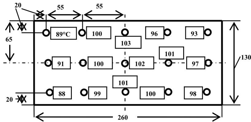
**Fig. 5** Temperature distribution in the sleeper cross section (size  $130 \times 260 \text{ mm}^2$ , MC = 34%, oven dry density  $480 \text{ kg/m}^3$ ) after traveling via applicator. MW power of 90 kW was supplied via 4 radiators (from top and bottom 25 kW each and 20 kW from every side, vector E orientation is perpendicular to the wood grain in all ports; speed—14 mm/s. Values in boxes—temperature in  $^{\circ}\text{C}$  measured in 15 points marked by circles)
