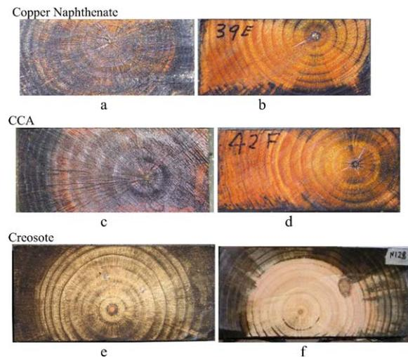
**Fig. 7** Sleeper cross section impregnated by preservatives after MW modification and controls. Copper Naphthenate: (a) MW treated—full cross section preservative penetration, (b) control, solution penetrates only to some small areas. CCA: (c) MW treated—full cross section preservative penetration, (d) control, only some areas are preservative treated. Creosote: (e) MW treated—full cross section preservative penetration, (f) control, only sapwood is preservative treated
