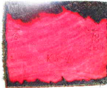
Figure 5. Karri timber sample with moisture content 70% after MW modification of the sample top and impregnation.
